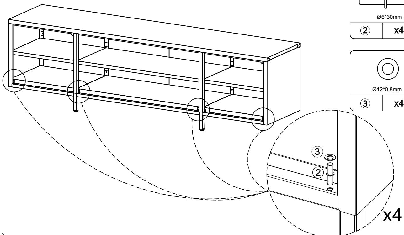
(10)- Attach (C1) &(C2)to pre-assembled unit as below shown.
